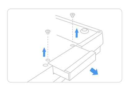
Step 4. Attach drive bracket to the new Solid-State Drive. Slide the drive into the bay until fully seated (Make sure to align the SATA plugs and solid state drive connectors)
